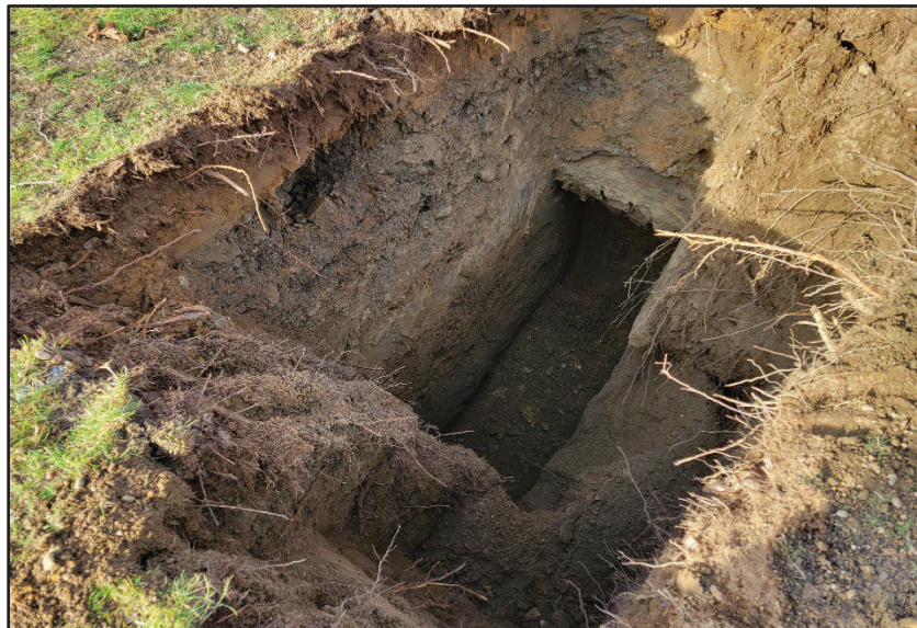
Image 2. Typical subsurface soil profile as observed in TP-2. Photo taken on 12-20-23.
